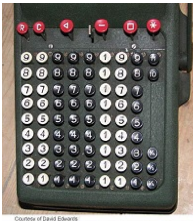
FIGURE 2. An £SD adding machine. Note the 3 keys on the lower right for farthings, the next row left with keys from 1 to 11 for pence, and the next two rows with keys from 1 to 19 for shillings. The remaining keys are for pounds.
